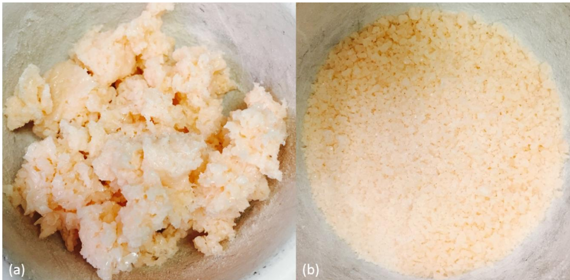
Figure 37. PS-PAESO polymer (a) before and (b) after grinding
