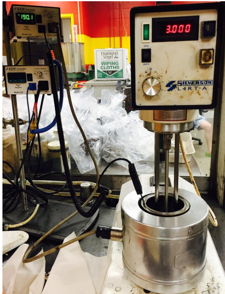
Figure 40. Shear blending at 3000rpm, 190°C
