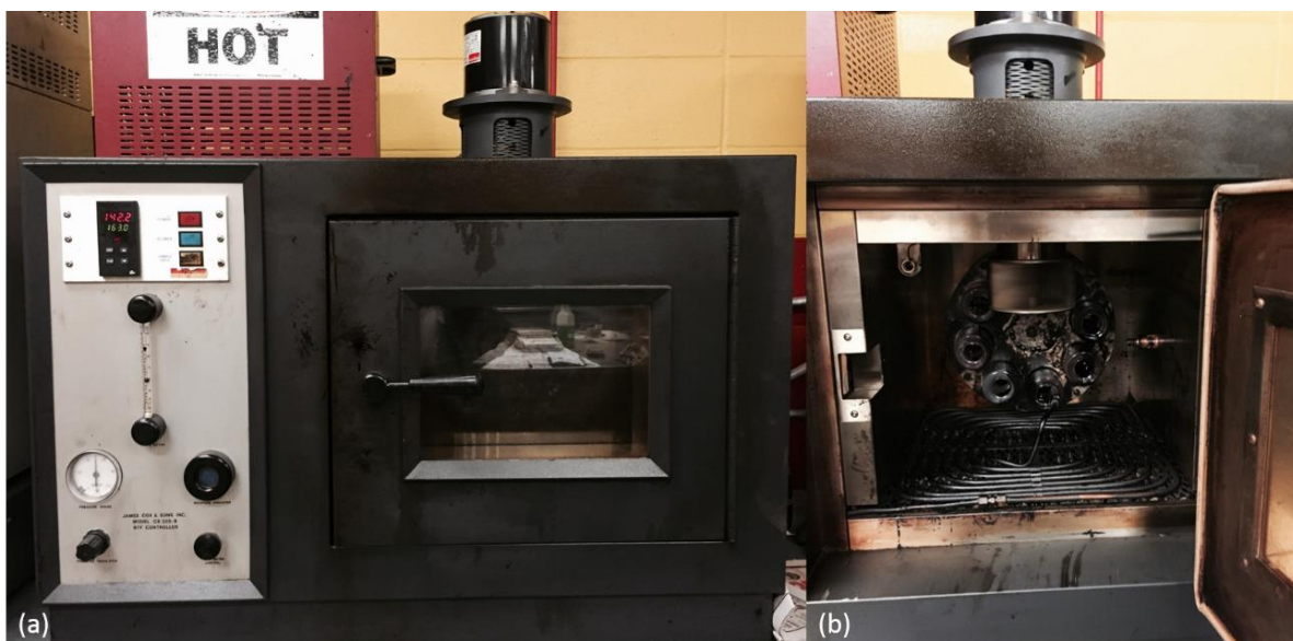
Figure 43. RTFO device (a) outside and (b) inside carriage
