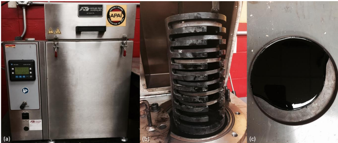
Figure 45. PAV (a) PAV device, (b) sample rack, and (c) PAV pan with 50\pm 0.5 g sample
