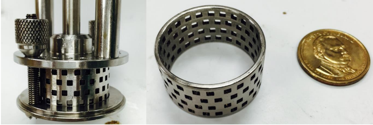
Figure 39. Shear head – square hole high shear screen
