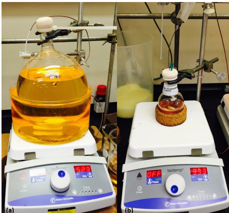
Figure 27. (a) Stirred blending and (b) purging under argon
