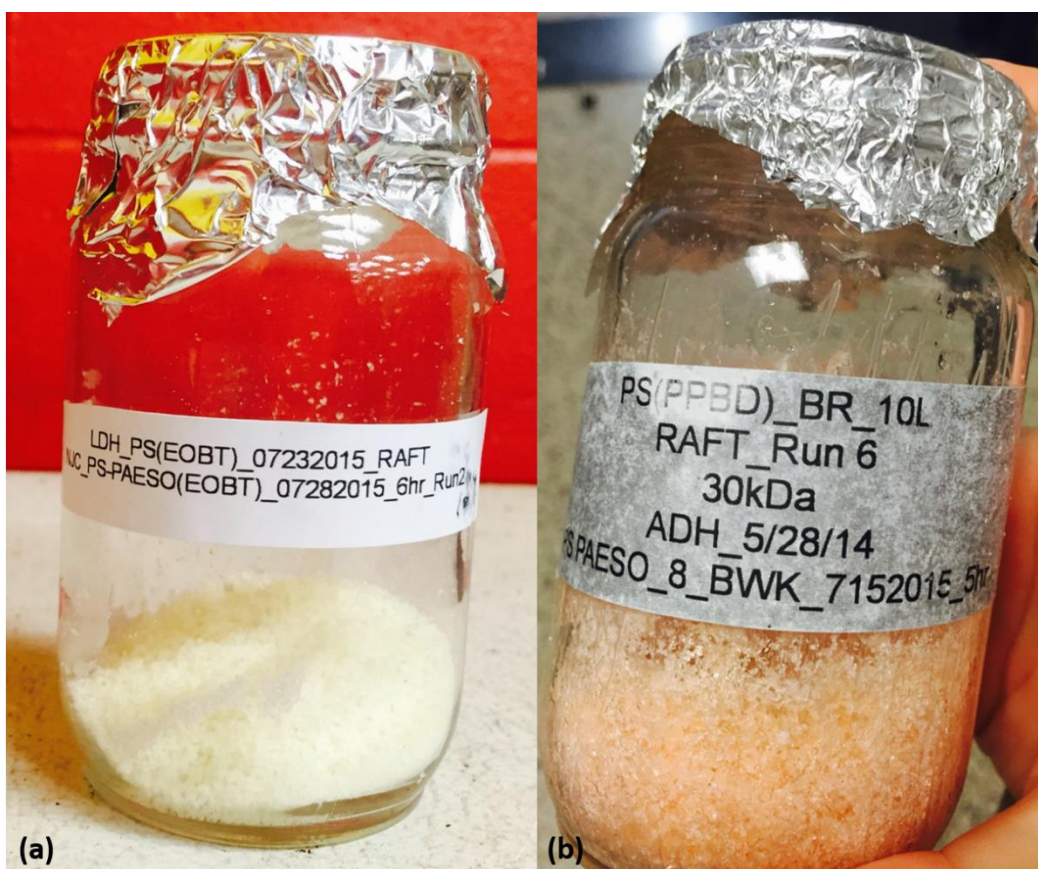
Figure 29. PS-PAESO with CTA of (a) EOBT and (b) PPBD
